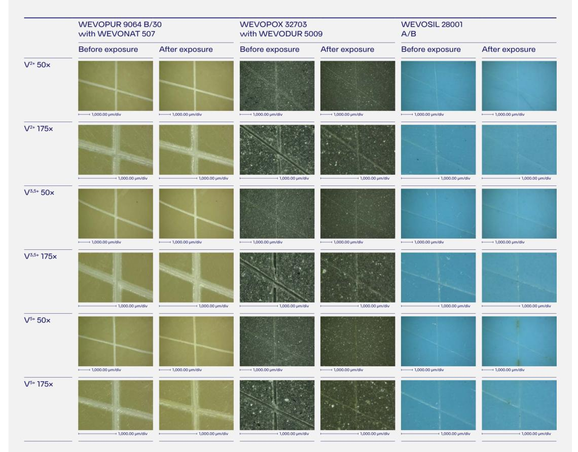
Optical analysis of test specimen with a light microscope at a magnification of 50× and 175× before and after exposure to the different electrolytes. The test specimens have been scratched by means of a cutter knife with a cross-shaped pattern. The more visible the cross pattern is and the sharper the lines after electrolyte exposure are, the more stable the polymer is against the electrolyte.
